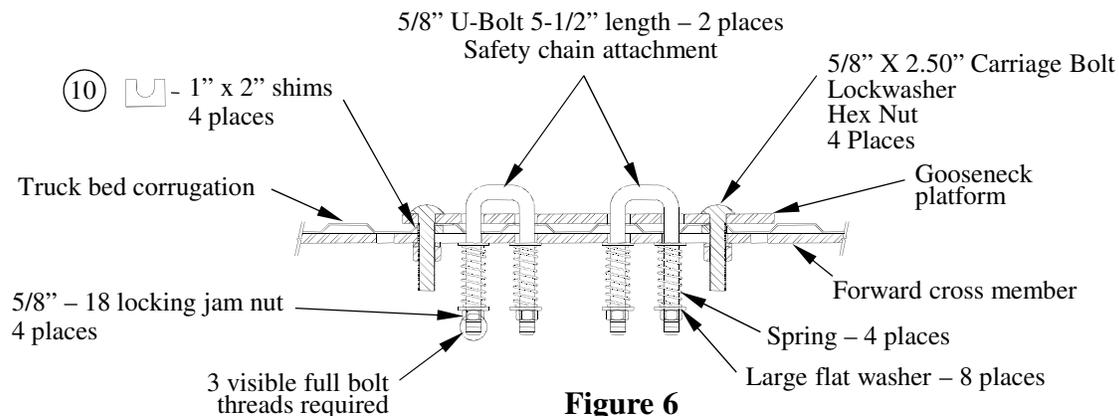
12. Before installing the 5/8" carriage bolts through the hitch, the U-Block shims must be placed between the hitch and the bed and between the cross members and the bottom of the bed (see Figure 6). These shims are necessary to prevent the bed corrugations from collapsing when the bolts are tightened.
