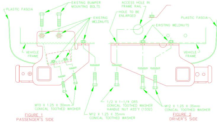
1. REMOVE TIE-DOWN BRACKET AT REAR END OF DRIVER'S SIDE FRAME RAIL. REMOVE TOW HOOK FROM REAR END OF PASSENGER'S SIDE FRAME RAIL. REMOVE TWO (2) BUMPER MOUNTING BOLTS FROM REAR END, OUTBOARD SIDE OF PASSENGER'S SIDE FRAME RAIL. RETURN TIE-DOWN BRACKET, TOW HOOK AND THEIR FASTENERS TO VEHICLE OWNER FOR REINSTALLATION IF HITCH IS REMOVED FROM VEHICLE. BUMPER MOUNTING BOLTS WILL BE USED FOR HITCH INSTALLATION.
