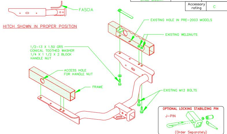
NOTE: SPARE TIRE MAY HAVE TO BE REPOSITIONED SLIGHTLY FORWARD TO AVOID CONTACT WITH RECEIVER TUBE.
