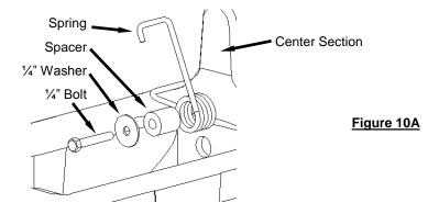
3B. The coil of the spring ( See Figure 10B) is facing the rear of the truck and wide hook sits over the center section casting as shown in Figure 10C Assemble and tighten 1/4" bolts into the thread holes in the casting.
