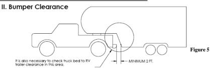
CAUTION: A minimum clearance between the bumper and trailer (Measured at the same height) of 2 ft. is recommended. Due to Vehicle and RV Trailer variations; it is necessary to check this clearance. If the clearance is less than the minimum, this can be done after installation by making a slow turn, in a controlled driving environment (i.e. closed parking lot, grass field, etc.) with the aid of an observer to watch for interference.
