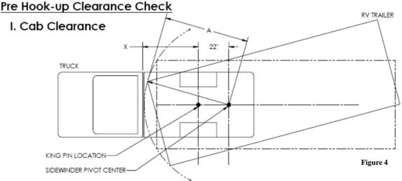
Measure Distance "A": From Center of Sidewinder™ pivot to farthest point on coach front cap.
