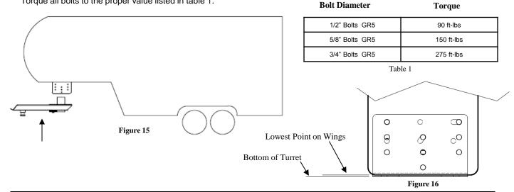
CAUTION: The bottom of the turret must extend below the lowest point on the wings to allow the arm to clear during pivot. (Figure 16)
