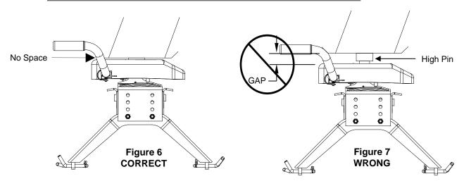
7. Place bail pin through bail pin holes in the handle and the base plate to make sure the hitch jaw is locked closed. IF FLAG BLOCKS HOLE FOR BAIL PIN, TRAILER HAS NOT BEEN PROPERLY CONNECTED TO HITCH. DO NOT TOW! Repeat above steps until trailer is properly hitched. (see Figure 8)
