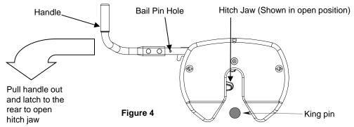
4. With handle in the open position (See Figure 4), back truck slowly into trailer. As king pin completely enters head, jaw will spring closed around king pin and handle will return to the closed
