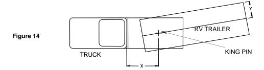
6. If a short bed pickup (less than 8 ft. but longer than 6 ft.) is to be used for towing, Cequent Performance Products recommends the trailer be equipped with an extended pin box to help gain additional truck - trailer turning clearance (See trailer manufacturer for options) (Figure 15). It also may be helpful to add a Square Tube or Round Tube Slider (Part # 30048 / 50008) for increased turning clearance for low speed, non-highway maneuvering.
