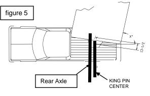
In this figure, the Kwik-Slide is positioned in the **Maneuvering Position**. Note that a 13-1/2" pin box extension has been used. The maneuvering Position should <u>only</u> be used at a low speed, when high maneuverability is needed!
