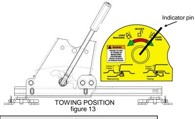
Leaf spring on latch cam keeps latch from disengaging. Hitch can not move rearward with latch engaged. Rearward load forces latch further into slot. Hitch can not move forward due to welded foot (see figures 1, 11 and 12).
