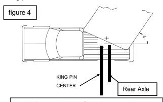
In this figure, the Kwik-Slide is positioned in the **Towing Position**, forward of the rear axle. Note that a 13-1/2" pin box extension has been used. This is the <u>only</u> position you should use when towing!
