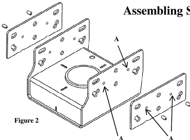
Position spacer plate (2) onto side of turret (1). Align holes (A) on spacer plate and turret. Install roll pin (3) into hole. Tap with hammer until flush with surface on the outside of turret.
