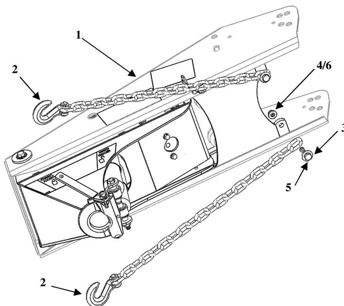
Locate Safety Chain Mounting Lugs On The Underneath Rear Of Your Goose Box. As Shown In Figure 1. Put Flat Washer Onto Bolt, Next Put Bolt And Washer Through Last Link In Chain, Then Position Bolt, Washer, And Chain Assy' Through Hole In The Mounting Lug, Secure With The Nut And Lockwasher.
