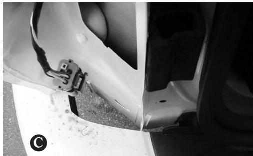
5. Disconnect the vehicle's Negative (-) battery cable. If not removed, remove the fuse from the **yellow** Fuse Holder (provided). After cutting the Fuse Holder wire **D**, attach the ring terminal and secure to the vehicle's Positive (+) battery cable. Connect the other end of the Fuse Holder to the **black** 12 ga. wire, using the **yellow** butt connector (provided) **E**.
