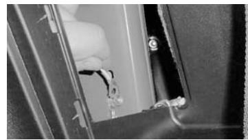
7. On passenger side, mount the T-Connector black convertor box in a out of the way place with the screw or cable tie provided and secure all loose wires with cable ties. Secure the remainder of the T-connector harness with the cable ties provided, to prevent damage or rattling and being careful to avoid any areas that would cut or pinch the wire.
