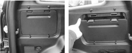
2. Partially remove the rear interior trim panels on both the driver and passenger side of the vehicle. Several trim panel fasteners will need to be removed to remove the panels. Set aside all items removed being careful not to damage parts.
