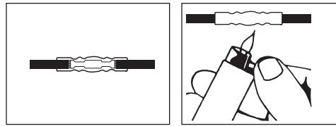
Apply heat directly to the splice, working from the center out to the edges, using a hot air gun or other source, until the tubing recovers and the adhesive flows. Allow to cool before inspecting splice and checking integrity.
